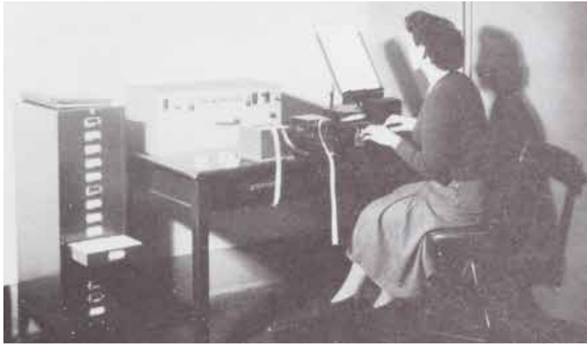
The library of tapes in which subroutines are punched is contained in the steel cabinet shown on the left. The operator is punching a program tape on keyboard perforator. She can copy mechanically tapes taken from the library on to the tape she is preparing by placing them in the tapereader shown in the center of the photograph.
